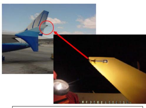
Pictured is the top portion of the fence (winglet) of aircraft 4846 (A320). This incident resulted in a crack in the fence, scratches, and a missing static wick.
