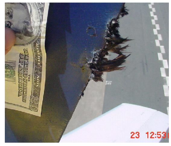
Common damage with no SRM repair
